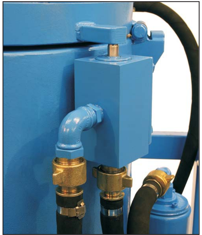
Safety interlock closed in operational position.
