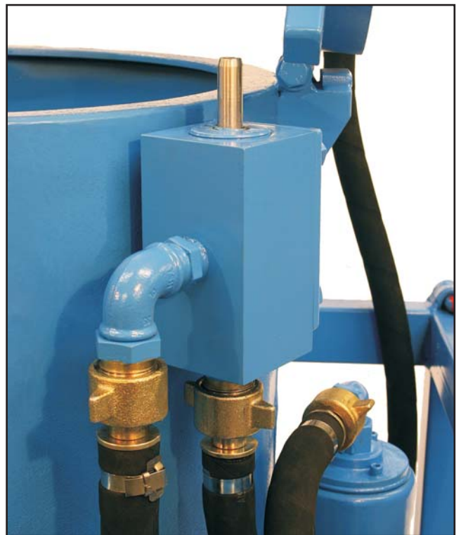
Safety interlock open, paddle operation disabled.
